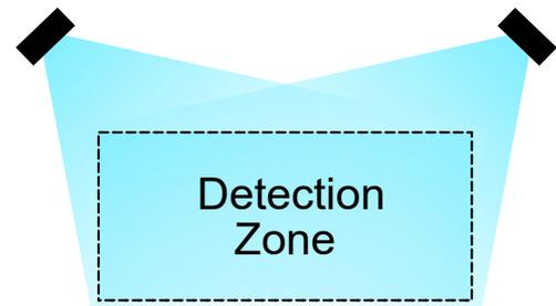
The minimum detection distance from our sensors starts at 1 m for static objects, for moving targets even at several centimeters. The maximum range for detecting human sized objects is up to 40 m. For bigger objects like trucks, the detection range is up to 200 m.
