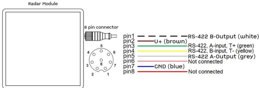
The radar system has the following interfaces:
