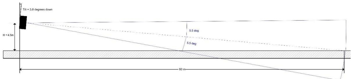
**Figure 1. Side view on an installation with a height of 4,5 m**
